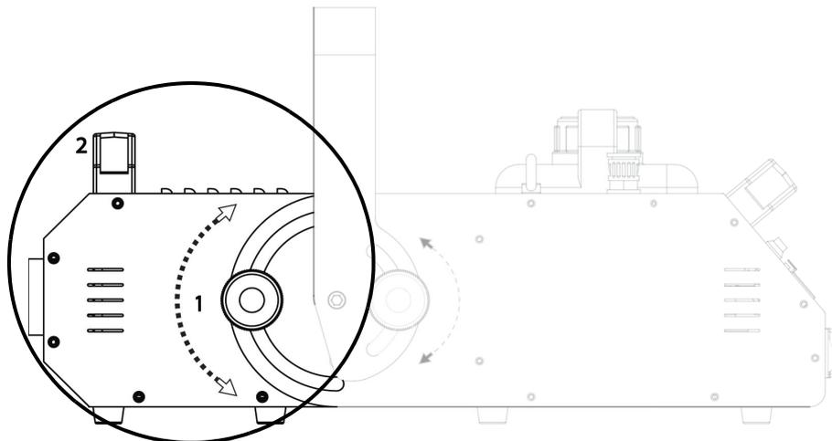
3. Loosen the angle adjustment knob<sup>1</sup>.
