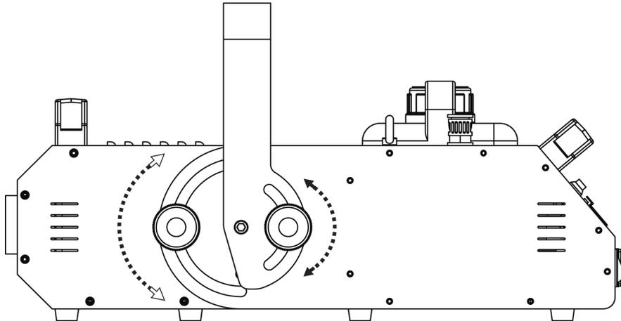
2. Use the bracket adjustment knob (black arrow in above image) to ensure horizontal hanging, if necessary.
