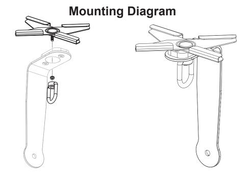
**Warning!** Prior to mounting, confirm the ceiling's load capacity with the facility manager. Scissor Clip load capacity: 3 lbs
