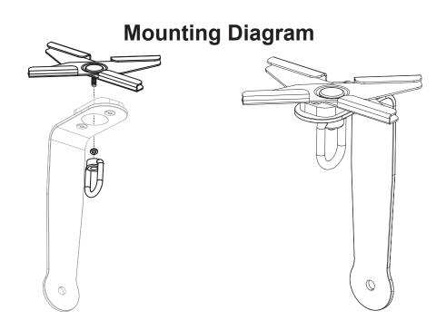
**Warning!** Prior to mounting, confirm the ceiling's load capacity with the facility manager. Scissor Clip load capacity: 3 lbs
