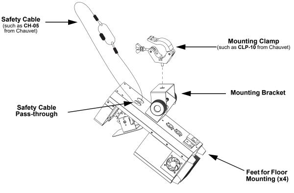
When using only one mounting clamp with this fixture, you must use a clamp with a captive bolt to prevent accidental loosening.
