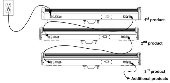
It is possible to link up to 12 COLORband PiX M ILS products on 120 VAC or up to 20 products on 230 VAC.
