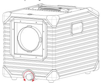
The next time the product is used, make sure to close the drain valve before filling the water reservoir. Cleaning the system prior to storage will help prevent any particles from condensing inside the pump or heater while not in use.
