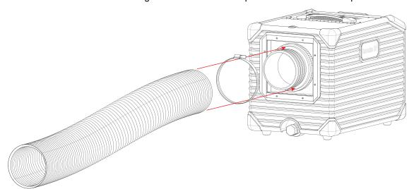
3. Ensuring the hose clamp is over both the hose and the hose coupler, turn the wingnut clockwise until the hose is secured to the coupler.
