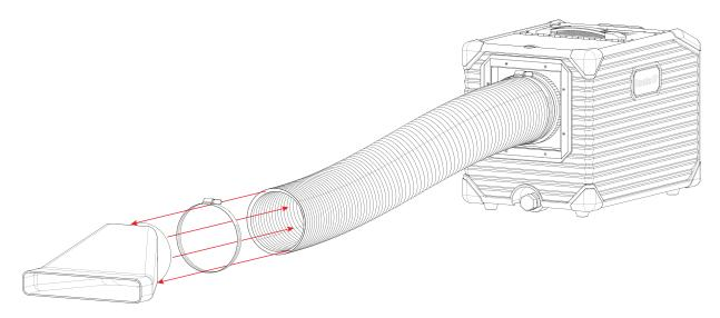
5. Ensuring the hose clamp is over both the hose and the floor nozzle, turn the wingnut clockwise until the hose is secured to the floor nozzle.
